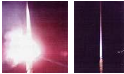
Tungsten rod evaporates within seconds
